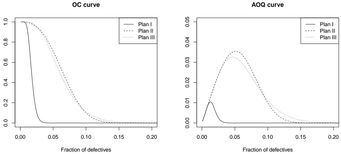
Figure 4: OC and AOQ curves of the Plan I ( $n_2 = 109$ ,  $k = 0.642$ ), Plan II ( $n_2 = 125$ ,  $k = 1.052$ ) and Plan III ( $n = 78$ ,  $c = 4$ ), designed to have risks  $\alpha = 5\%$  and  $\beta = 10\%$ , when  $AQL = 2.5\%$  and  $LTPD = 10\%$ .
