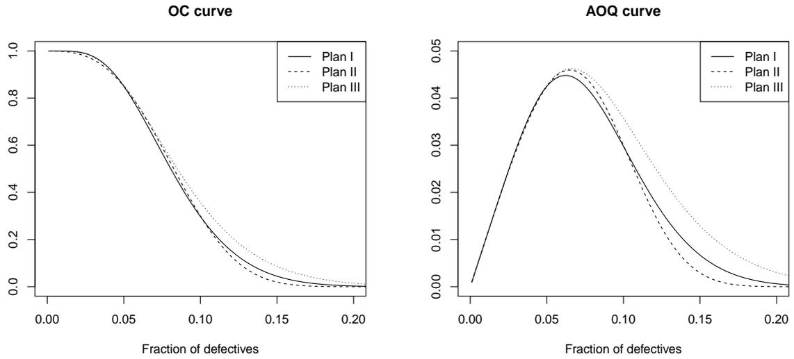
Figure 3: OC and AOQ curves of the Plan I ( $n_2 = 16$ ,  $k = 1.213$ ), Plan II ( $n_2 = 81$ ,  $k = 1.204$ ) and Plan III ( $n = 55$ ,  $c = 4$ ), designed to have risks  $\alpha = 15\%$  and  $\beta = 30\%$ , when  $AQL = 5\%$  and  $LTPD = 10\%$ .
