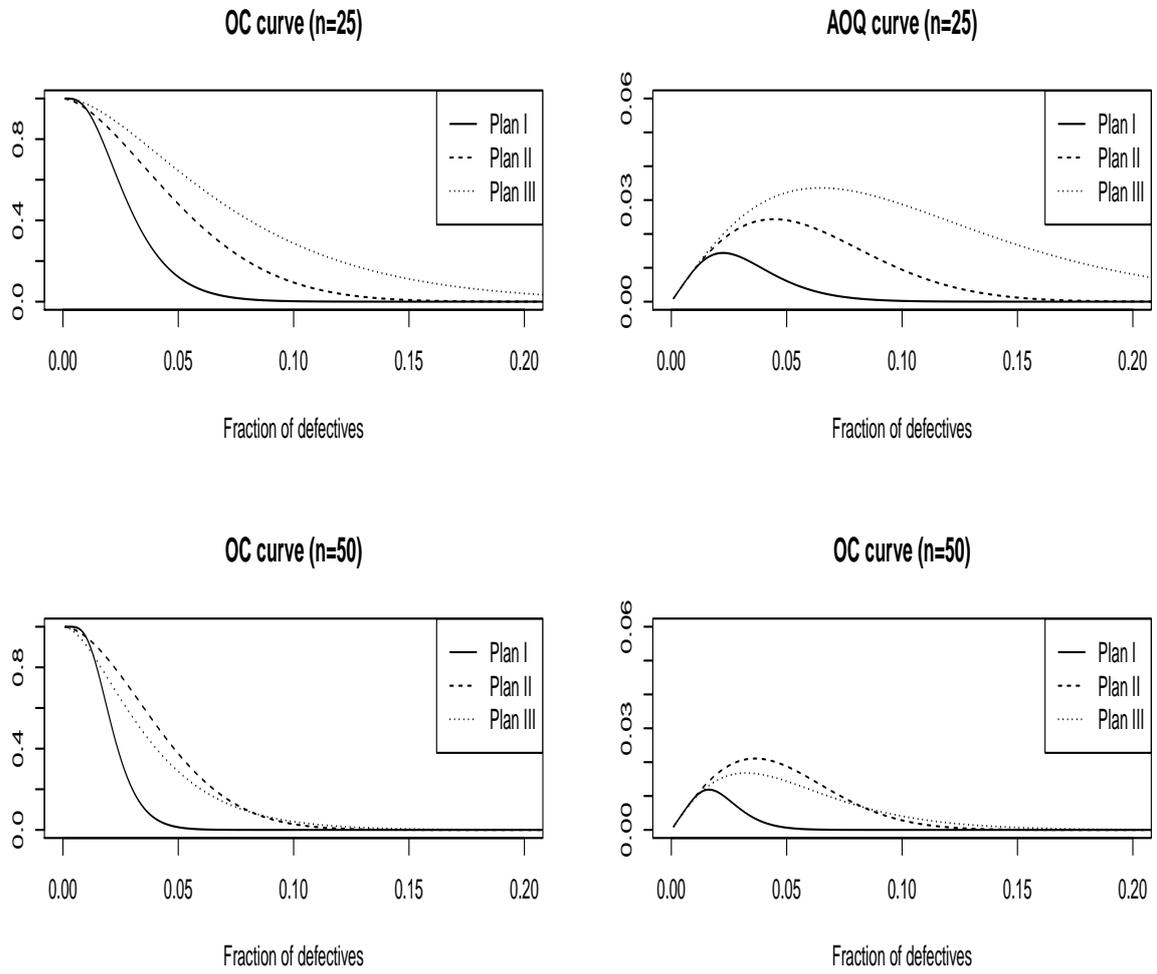
Figure 6: OC and AOQ curves of the sampling plans designed to have an  $\alpha$ -risk 5% when  $AQL = 1\%$
