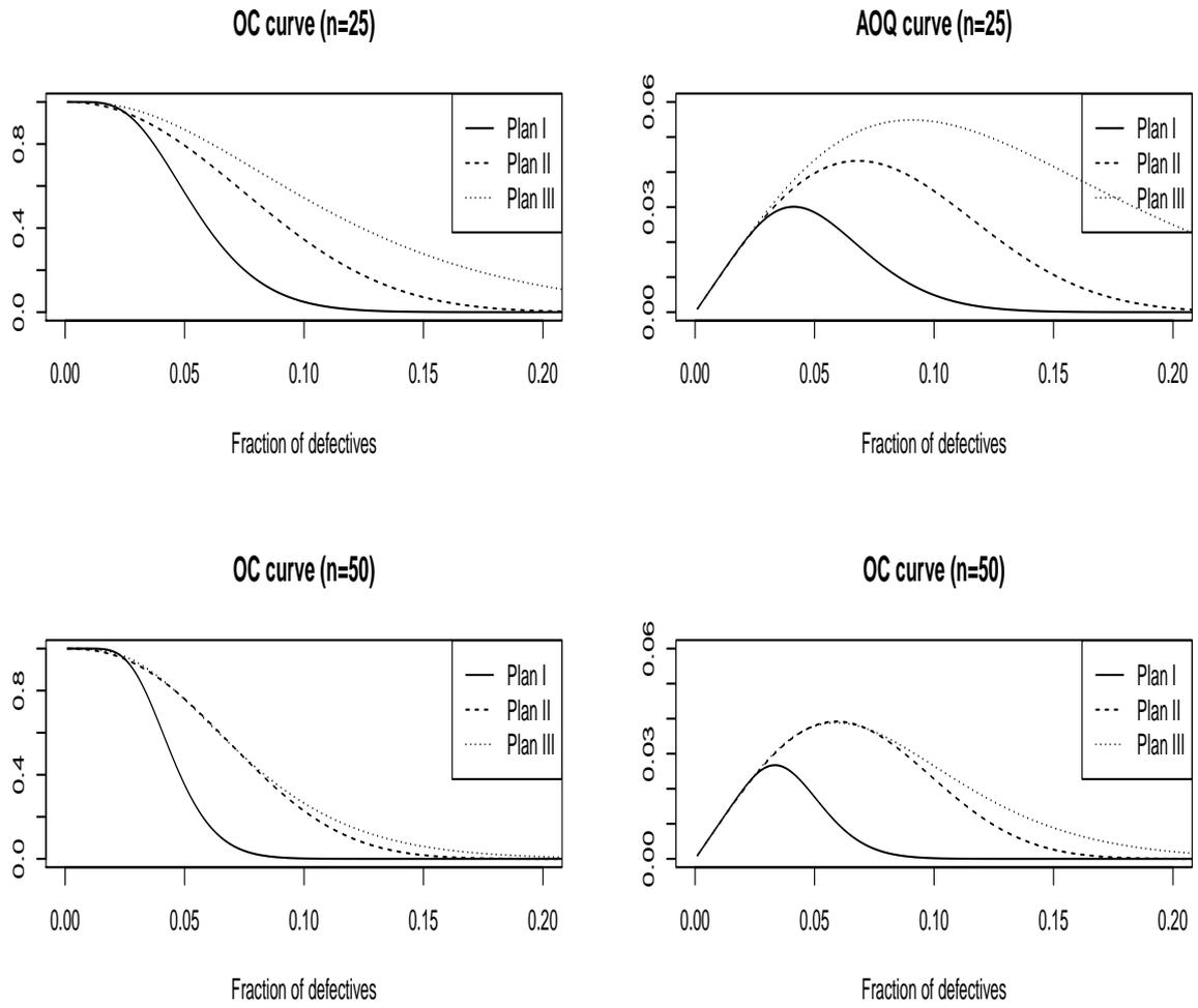
Figure 5: OC and AOQ curves of the sampling plans designed to have an  $\alpha$ -risk 5% when  $AQL = 2.5\%$
